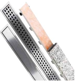
The Schluter®-KERDI-LINE is a low profile linear floor drain specifically designed for bonded waterproofing assemblies. KERDI-LINE can be installed adjacent to walls or at intermediate locations in showers, wet rooms, and other applications that require waterproofing and drainage. The floor can be sloped on a single plane to KERDI-LINE, which enables the use of large-format tiles and creates interesting design opportunities.
