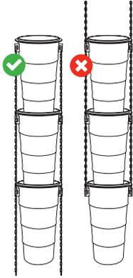
The chute chains should always be hanging down, never upwards.
