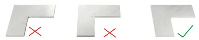
To make the corners of the cut-out, drill them with a bit with a radius of > 3 mm.
