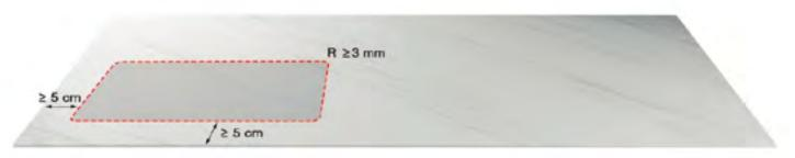
A bigger radius will ensure a higher structural resistance. In contrast, angles with no radius create a stress point on the surface. NEVER LEAVE 90° ANGLES.
